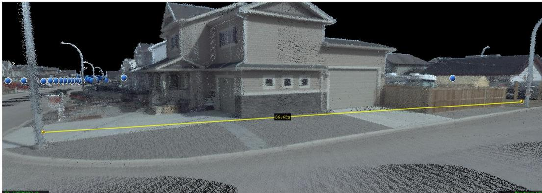
3D Point cloud captured from LiDAR
