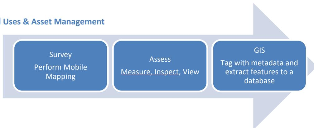
A Geographic Information System (GIS) is a solution for capturing, storing, manipulating and presenting all types of geographic data. A terrestrial mobile map is the easiest way to capture data to populate a GIS system with a local survey, as it has the necessary resolution, definition and accuracy to identify and locate surface assets.
